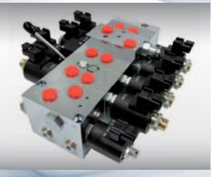
Up to 50 l/m (inlet flow) Direct acting proportional solenoids Load sensing configuration with pressure compensation on each single section Meter-in control available
